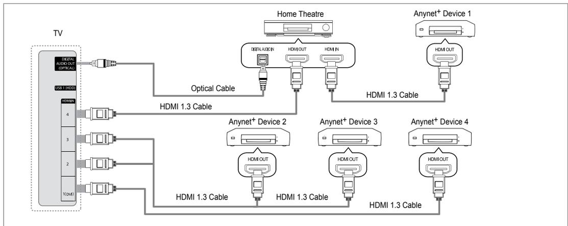
1. Connect the **HDMI IN (1(DVI), 2, 3 or 4)** jack on the TV and the **HDMI OUT** jack of the corresponding Anynet+ device using an HDMI cable.
