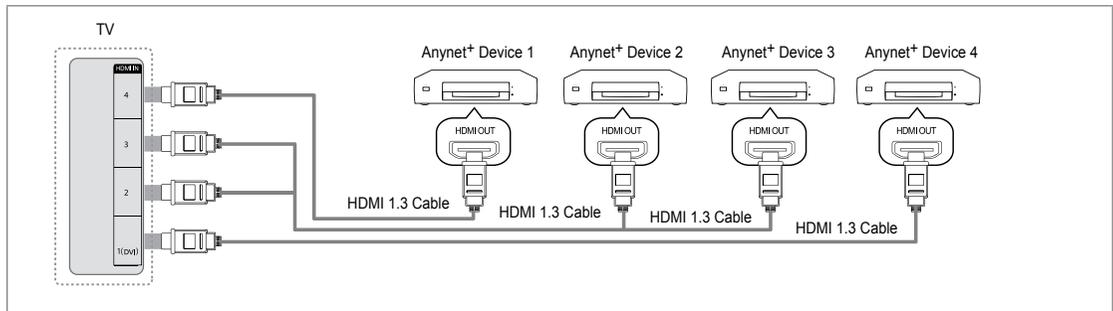
1. Connect the **HDMI IN (1(DVI), 2, 3 or 4)** jack on the TV and the **HDMI OUT** jack of the corresponding Anynet+ device using an HDMI cable.
